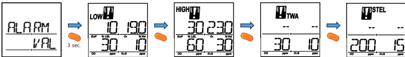
Press the KEY button (
