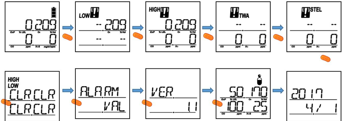
The displays in ten different modes as above are shown in the measuring mode every time when you press the KEY button( ).
