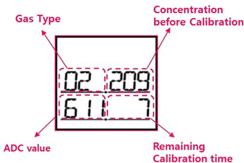
**Initial Standard gases concentration for calibration**
