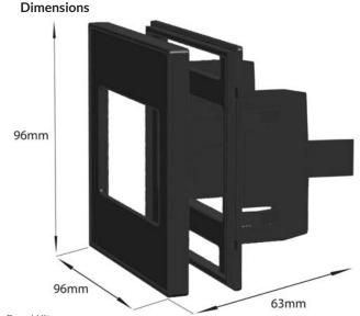
Panel Kit: Height: 96mm Length: 96mm Depth: 63mm Face Hole: Height: 41mm Length: 71mm
