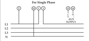
It is recommended that the wires used for connections to the instrument should have lugs soldered at the end. That is, the connections should be made with Lugged wires for secure connections. The Maximum diameter of the lug should be 7.0 mm and maximum thickness 3.5 mm.
