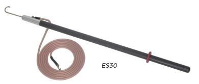
The ES30, ES50 and ES100 earthing sticks are designed for earthing the high voltage connection after ac testing in accordance with EN50191. The earthing sticks consist of a hooked earth connection mounted on an insulated handle with a 5m earth lead. The earth lead insulation is clear silicone allowing the conductor to be easily inspected, and is terminated in an M6 hooked crimp.
