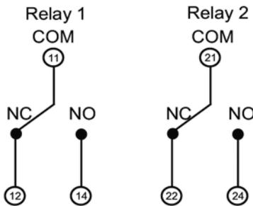
Note- Relay Contacts are shown in power off condition
